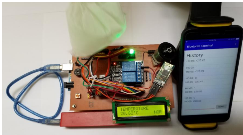
Figure 13 The photograph of normal (between 20°C and 30°C) temperature range of the system
