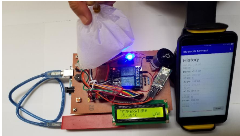
Figure 12 The photograph of Low (between above 5°C and 20°C) temperature rang of the system
