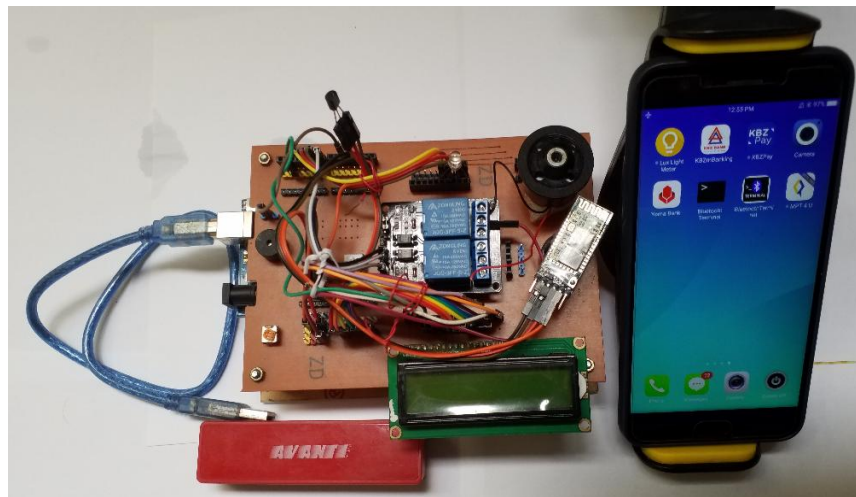
Figure 10 The photograph of the assembly of the temperature indicator circuit
